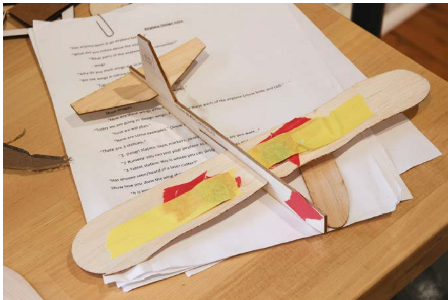
Design Lab creation, airplane wings designed on tablets and cut on laser cutter
